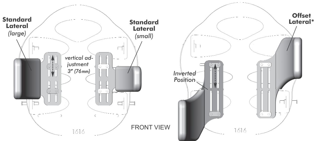
**\*note:** offset laterals may also be mounted in the inverted position (as shown) to provide extended support
